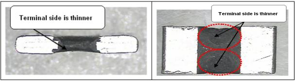
8.3.2 When customer performs wave solder process shall take note on the dispensing gap. If the gap between two dispensing is over, the red-glue will not adhesive the resistor body and be dropped out (as photo 1). Therefore, we suggest customer to narrow down the dispenser gap (as photo 2), or dispenser on the body center (as photo 3)
